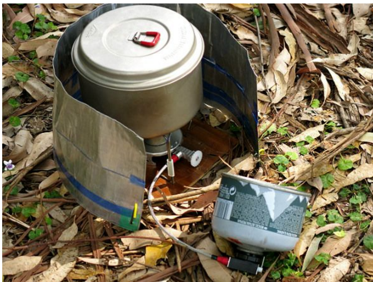
1.5 L MSR Titan pot sitting on pot stand 75 mm high on light 3-ply base board, with a windshield which is really higher than needed around it.
